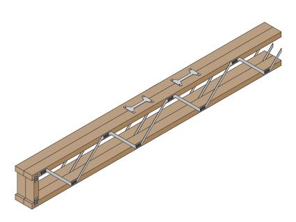
5. Floors should provide lateral restraint to all walls running parallel to them by means of 30mm x 5mm galvanised or stainless steel restraint straps at 2m centres.
