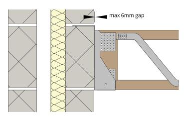
4. Double joists should be fixed as per the manufactures design. This may for example be with a propriety clip fixed at specified centres. It is important to ensure that the work on site is in accordance with the manufacturers design.
