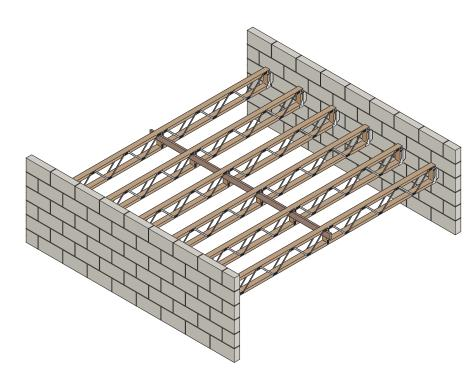
7. Perimeter noggins are required at the perimeter of joists to support the floor decking above and to create a stronger and more rigid frame. They should be fitted with Z-clips.
