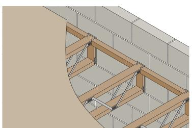
8. Where studs above run parallel to joists, they should be supported on multiple joists or a row of noggins. Where they are supported on noggings, the soleplate for the stud should be fixed into the noggin. Where you see multiple fixings through the decking in a row, it may be due to a stud above not being supported or fixed into the noggins.
