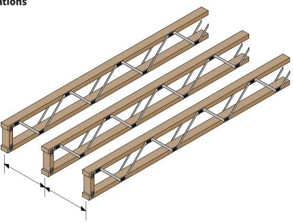
2. Joists are designed with a specific top and bottom chord, the joists should be marked to indicate which the top chord is, if in doubt speak to the manufacturer.
