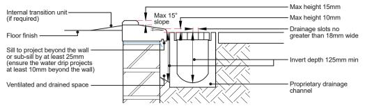
These illustrations show accepted practice for forming a weather resistant threshold detail and may not indicate the full extent of insulation requirements to meet relevant Building Regulations.
