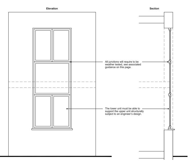
Fixing should allow for differential movement if in a timber framed building as well as suitability to join one frame to the other. Fixings must also meet the requirements of BS8213: 4 for spacing requirements with particular emphasis on the side and tops.
