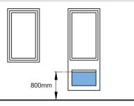
If permanent protection is provided in the form of fixed guarding, there is no requirement for the glazing itself to be of a special type. Permanent protection may take the form of railing or barriers and should:
