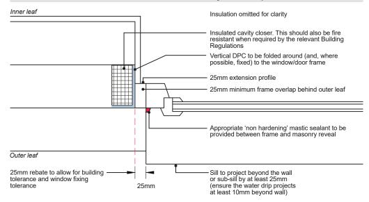
When installing window/door frames in a checked rebate, allow for the frame to be deeper:
