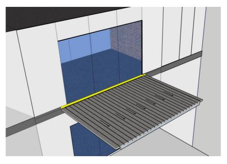
Figure 2 – Yellow denotes upstand. Details relating to non-combustible pedestrian surface and guarding omitted for clarity.
