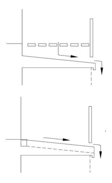
Figure 1 - Examples of acceptable drainage approaches for projecting balconies.
