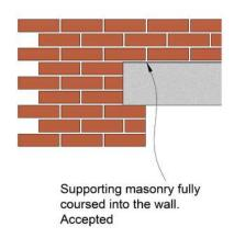
Figure 15: Correct method of brick bond around lintels
