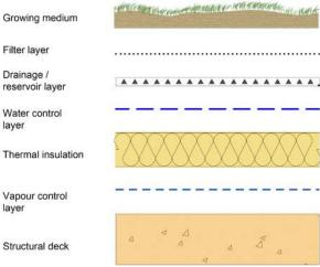
Figure 1: Extensive green roof - warm roof system (section)
