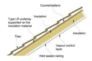
Figure 9: Warm roof construction (vapour breathable underlay)
