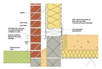
Figure 3: Sole plate / foundation junctions
