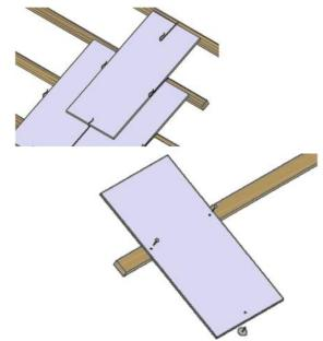
Figure 13: Fixing slates
