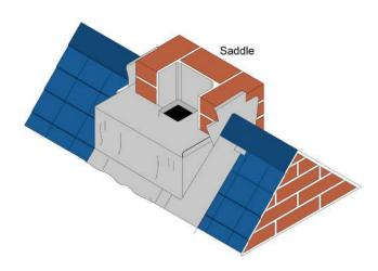
Figure 3: Flashings to chimneys at ridge
