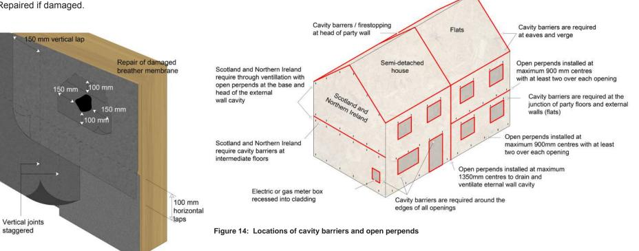
Figure 13: Lapping and repair of breather membrane
