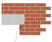
Supporting masonry not fully coursed into the wall. Not accepted
