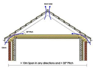
Figure 3: Duo-pitch roof B
