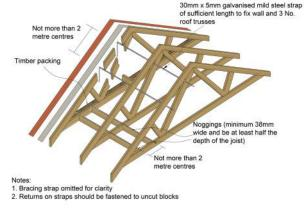
Figure 7: Lateral restraint to gable wall via roof trusses
