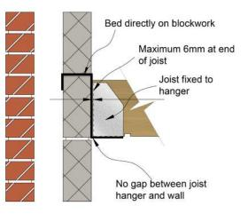
Figure 3: Typical restraint type joist hanger
