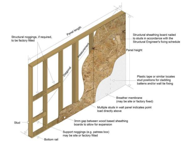
Figure 4: Typical wall panel
