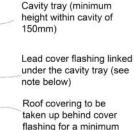
Tilting fillet to support roof covering at junction
