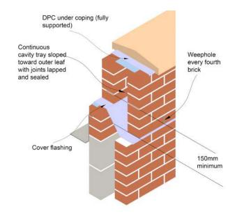
Figure 21: Parapet wall detail
