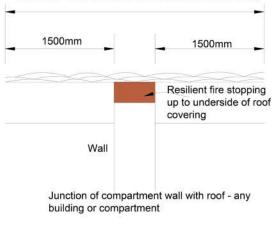
Figure 13: Typical fire stopping details
