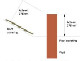
Junction of compartment wall with roof - any building or compartment
