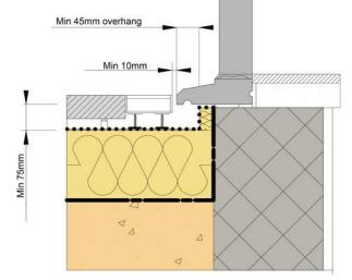
Figure 6: Details - Principles – Upstand at door access - Inverted warm deck roof Figure 7: Details - Principles – Upstands to decking and paving finishes, (e.g. balcony parapet) – Warm roof.
