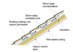
Figure 8: Warm roof construction (vented battens)
