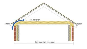
Figure 2: Duo-pitch roof A
