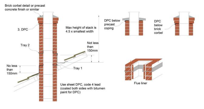
Figure 1: Typical chimney details
