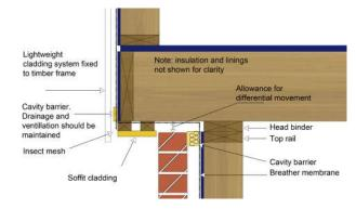
Figure 23: Differential movement at cantilevered overhang
