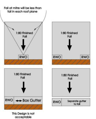
Figure 4: Drainage layout options
