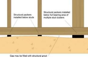
Gap may be filled with structural grout or sealant to maintain air tightness
