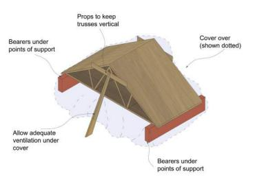
Figure 2: Site storage of trusses
