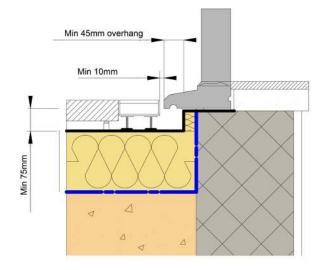
Figure 5: Details Principles – Upstand at door access - Warm deck roof – Level threshold
