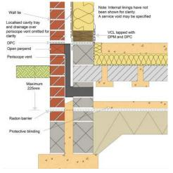
Figure 5: Possible gas membrane detail
