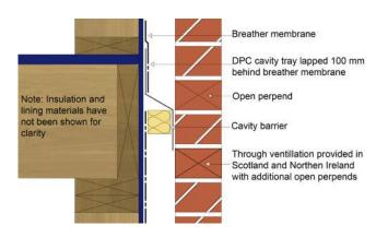
Figure 15: Cavity tray above horizontal cavity barrier
