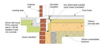
Figure 2: Typical level threshold suspended concrete slab
