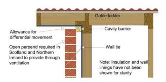
Figure 22: Differential movement at verge
