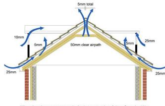
Where there is no cross communication between each roof slope, 5mm should be provided on both sides of the ridge
