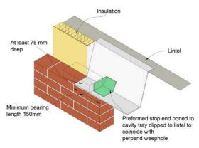
Figure 18: Stop end to cavity tray
