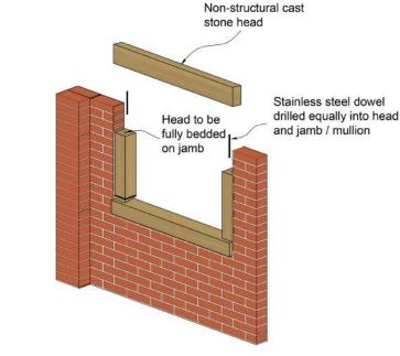
Figure 25: Stone jamb and mullion, fixing to walls
