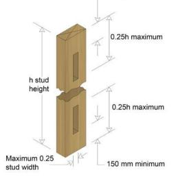
Drilling on centre line only. Hole diameters not greater than 0.25 stud width and hole centres not closer than 4d (d = hole diameter)
