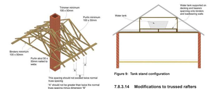
Figure 8: Roof trusses trimming around a chimney
