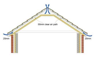
Figure 5: Duo-pitch roof with sloping ceilings
