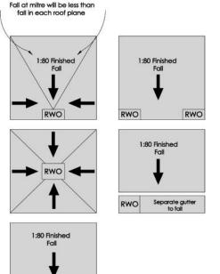
Figure 4: Drainage layout options
