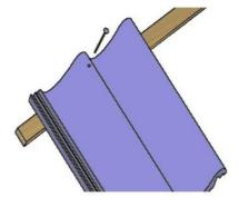
Figure 11: Nailing tiles to battens
