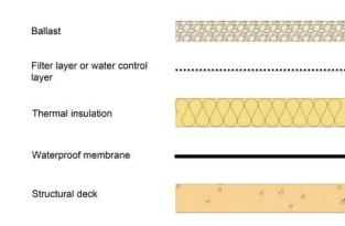
Figure 2: Inverted warm roof (section)
