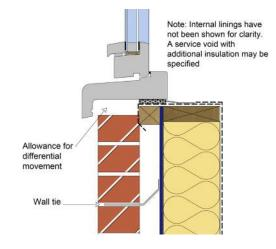
Figure 20: Differential movement gap under sill
