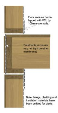
Figure 12: Typical floor zone air tightness detail
