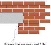
Supporting masonry not fully coursed into the wall. Not accepted
