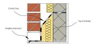
Figure 19: Stop-end in relation to cavity tray and lintel
