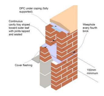
Figure 21: Parapet wall detail
