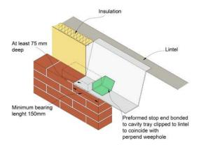
Figure 18: Stop-end to cavity tray
