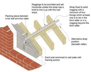
Figure 5: Lateral restraint strap to gable wall
