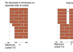
Figure 12: Typical corbelling arrangements
