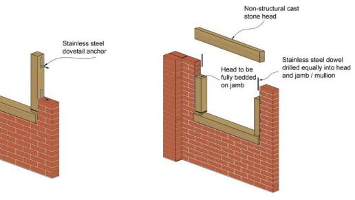
Figure 25: Stone jamb and mullion, fixing to walls
