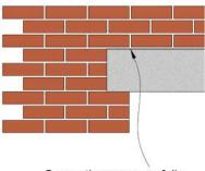
Supporting masonry fully coursed into the wall. Accepted
