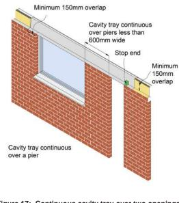
Figure 17: Continuous cavity tray over two openings and a small pier
