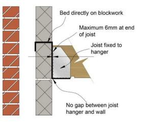
Figure 3: Typical restraint type joist hanger
