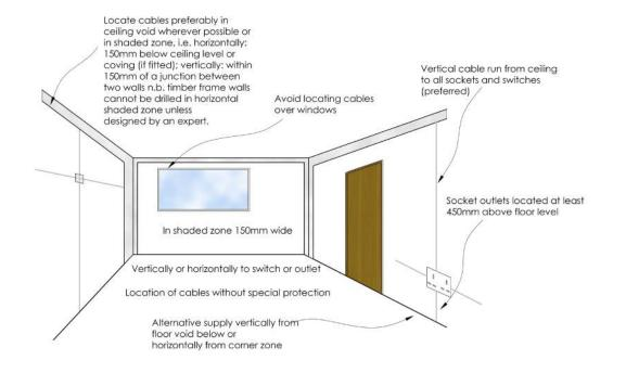
Figure 8: Location of cables without special protection
