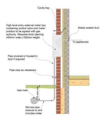
Figure 12: Gas service pipes
