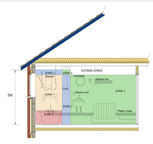
The protective conductors of all power and lighting points within zones must be supplementary bonded. The bonding connection may be to earth terminal of a switch or accessory supplying equipment.
