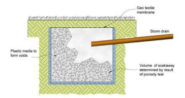
Figure 3: Typical soakaway design
