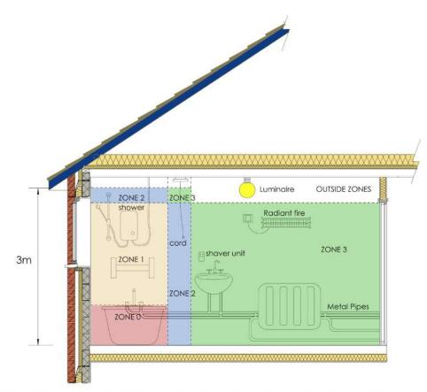
The protective conductors of all power and metal lighting points within the zones must be supplementary bonded to all extraneous conductive parts in the zones including metal waste, water and central heating pipes, metal baths and shower basins.
