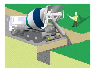
Figure 6: Ready mixed concrete
